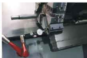
Boring bar concentricity inspection
