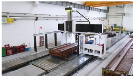
ZAYER gantry milling center-Spain(25m)
