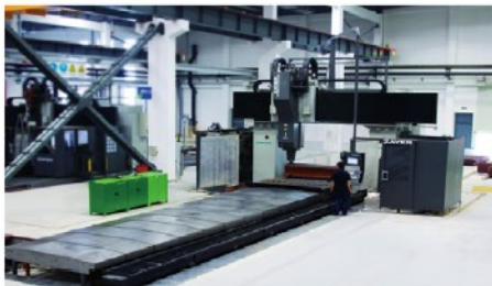
ZAYER gantry milling center-Spain(10m)
